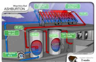
We recently completed a monitoring callibration on a 1 year old SolarPeak Dairy Solar system in Ashburton. The system comprises 2 x 700 litre dairy solar cylinders and 4 x 30 tube collectors using a unique hydraulic design by Glenn Harvey of SolarPeak.
